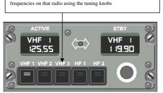
Pressing radio select button displays active and standby frequencies
